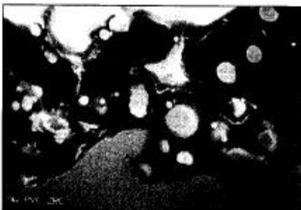
Fig. 4: Photomicrograph of unexposed film of 22764I. Note the presence of isolated zinc particles in electrically insulative resinous matrix.
